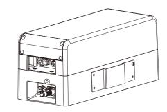
After the power cable has been correctly connected, and all RS485 communication cable (please refer to section 4.5.2) and ground wires (please refer to section 4.5.4) are correctly connected, lock the terminal box\_large(L) to the out side of BMS and battery module on the left with M4 screws(N).
