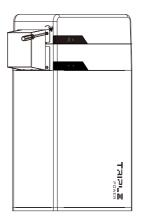
On the right side of BMS, after the charging cables (please refer to section 4.5.5) and CAN communication cable (please refer to section 4.5.3) are correctly connected, screw the terminal box\_small (J) with M4 srews and lock the terminal box cover (K) also with M4 screws. On the right side of battery module, screw the terminal box\_medium\_right (I1) with M4 screws and lock the terminal box cover (K1) in the same way as BMS. Please see the installation diagram on the right.
